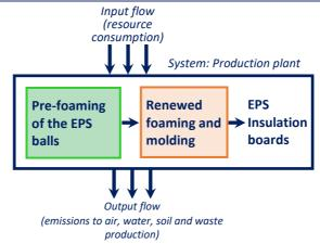
Simplified representation of the processes in the manufacturing phase of swissporEPS insulation boards (phases A1 -> A3)
