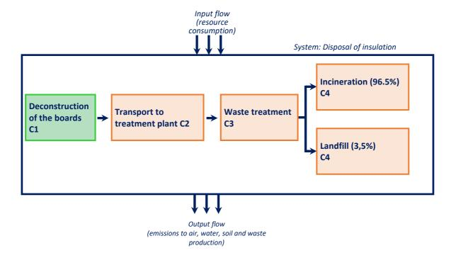
Simplified scheme of the disposal processes (phases C1 -> C4)
